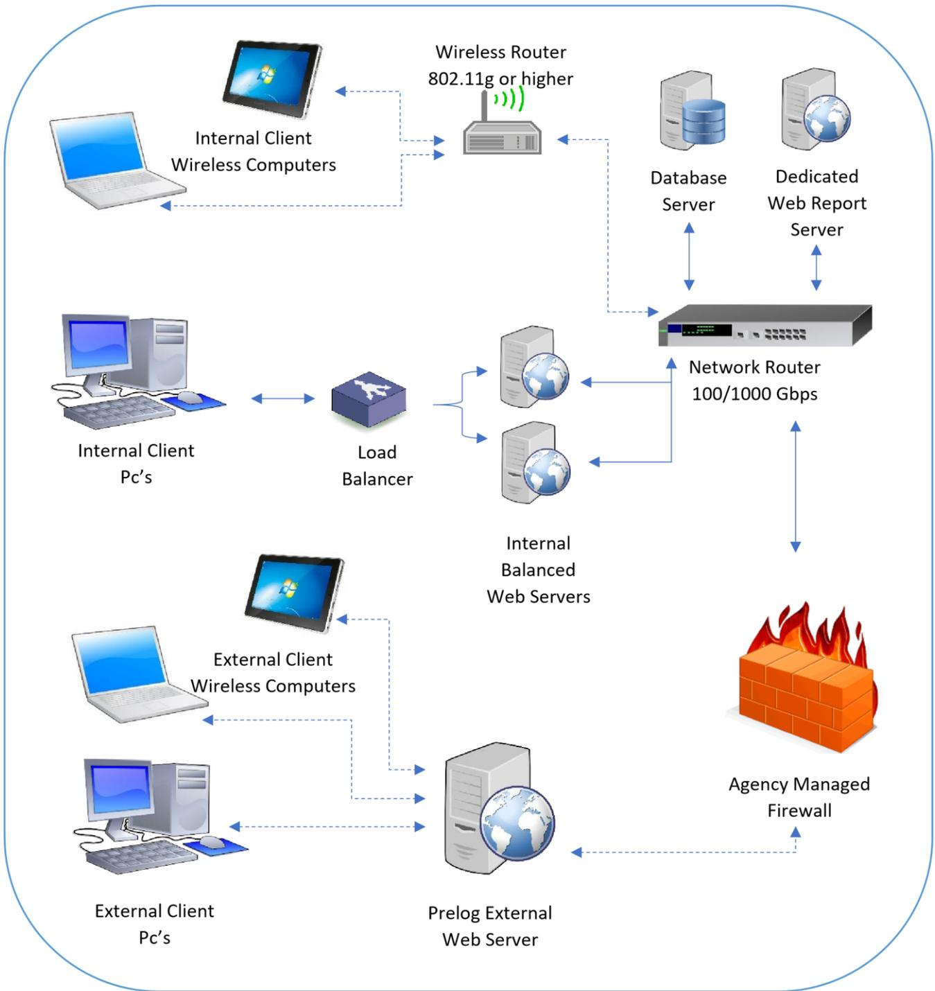
Sample Scaled Schematic Diagram
